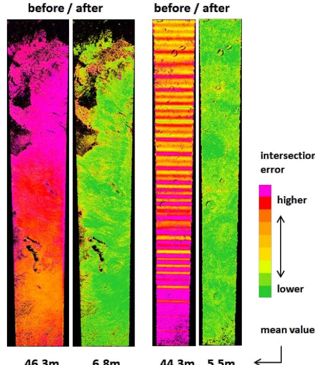
**Improvement of intersection error by photogrammetric adjustment: time-dependent corrections to orientation angles pitch, roll and yaw.**
